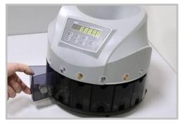
It is very easy to remove a full tray. To continue the counting, it is necessary to place the empty tray back into the machine and then press the «START» button.
