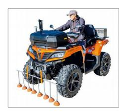
The Scout VGS 4500 measuring unit is operated and monitored using a tablet PC. The software was developed and programmed by Schütz GmbH Messtechnik specifically for the system. It displays the measurement route in real time, automatically records and logs each leak. In the scope of delivery: a worldwide overview map (OSM) is already included. Furthermore, a map of the gas pipeline network to be inspected can be read in.
